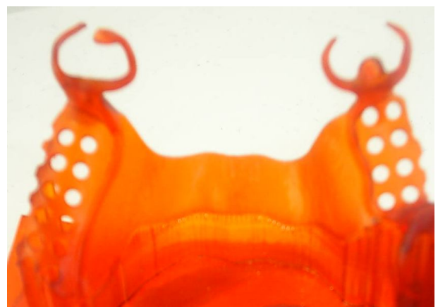
Fig.3 Basis for dental prosthesis made of PMMA by selective laser sintering (SLS).
